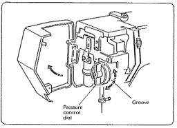
The pressure control dial is located inside the face cover plate.
